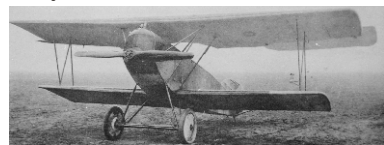
A typical OAW built Fokker D.VII. The nose giraffe pattern, the two tone painted wheel disks and the half and half separated green/mauve axle cover are visible. (Albatros/PL Gray Collection-used with permission)
