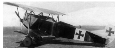
An early Fokker D.VII with Mercedes D.IIIa engine in the typical Fokker streaked finish (Albatros/PL Gray Collection-used with permission)
