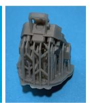
3D printed resin parts are super detailed and accurate however the resin can be brittle and snapping the parts from their printing supports will nearly always leave a 'divot' in the part. This divot may or may-not require filling depending on its location on the finished part. CA or filler can be used to repair.
