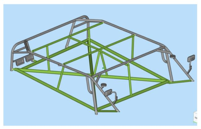
**Remove** the green coloured parts as shown in the diagram accordingly.
