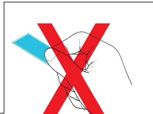
1. Separate the etched components from their frames on the protective paper. Removal from the paper is done only after separation of the parts from the frames.
