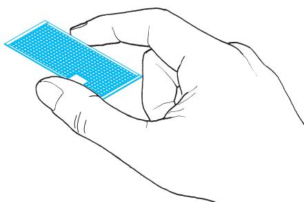
2. Do not inadvertently place etched components on an unwanted surface. Attempts to remove will result in damage to your part.
