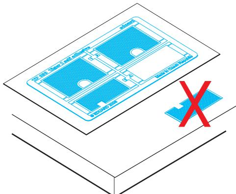
5. Lightly place the component in the desired location and position. Adjust as required. The component will be permanently affixed when pressed onto its intended location, its location can be adjusted.
