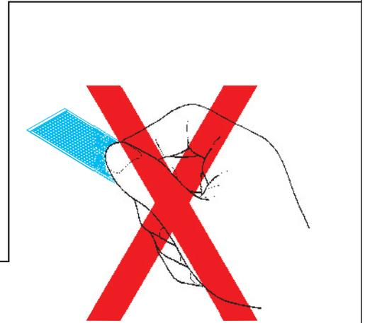
1. Separate the etched components from their frames on the protective paper. Removal from the paper is done only after separation of the parts from the frames.
