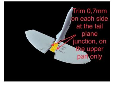
This step ensures there is a minimal gap on the underside of the tailplane.
