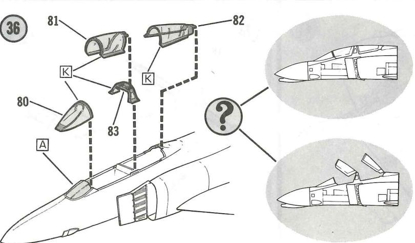
CANOPY DETAIL—MASK ENTIRE CANOPY WITH A DULL FINISH ACETATE MENDING TAPE. CAREFULLY CUT THE TAPE FROM AREAS TO BE PAINTED. PAINT THE EXPOSED PARTS AND ALLOW TO DRY. REMOVE THE REMAINING TAPE.
