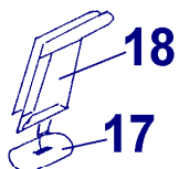
Underside VHF [FM] Radio Antenna - shown inverted
