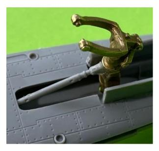
Pictures show the kit parts attached to the brass, for this PVA glue or super glue is recommended.
