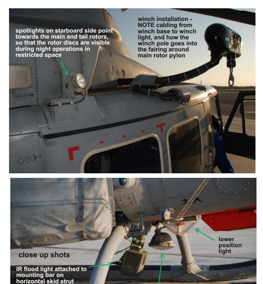
downward pointng spotlight attached to mounting bar on horizontal skid strut
