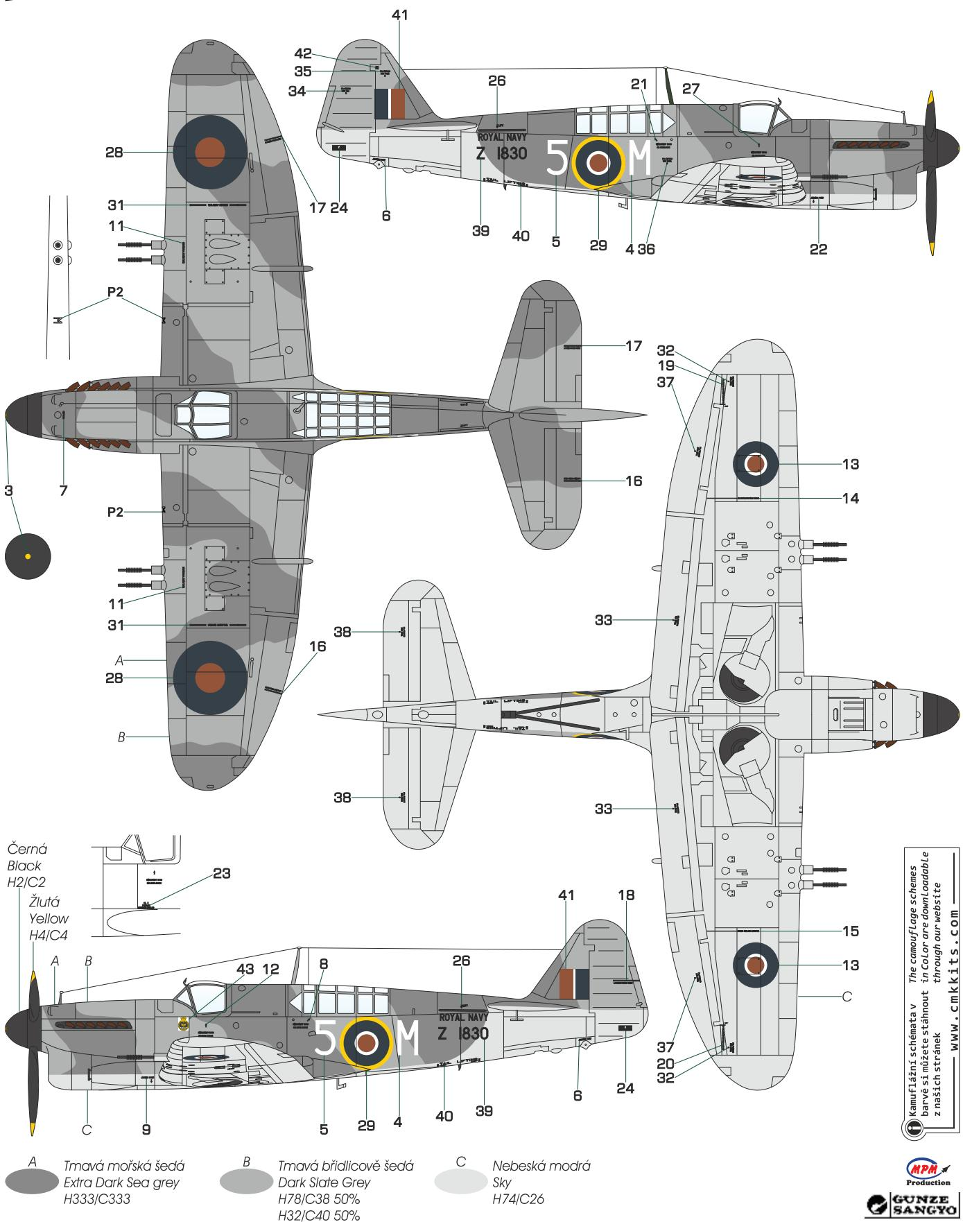
Fairey Firefly Mk.I, 5M/Z1830, FAA No. 1770 Squadron, HMS Indefatigable, July 1944. This machine participated in operation in Mascot – the attack on Tirpitz. This was a premier deployment of both HMS Indefatigable and Firefly fighters. The aircraft featured early windshield and cannons without the aerodynamics fairings; in fact this was the first Firefly Mk.I production machine.
