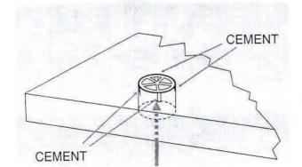
First, cover the surface of deck with No 500 primerl. (Attention: Surface side is the one which have lines incised.)
