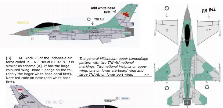
[C] F-16B Block 15 OCU of the Indonesia air force TS-1602 serial 87-0722 is an early F-16. This second hand jet has the standard U.S paint scheme of FS36270 lower surfaces and FS36375 on forward upper surfaces , part of intake, belly fins and tail and FS36118 on upper surfaces. Flag on tail on both sides.
