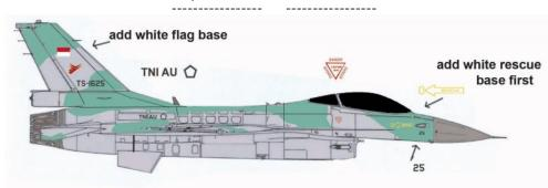
[A] F-16C Block 25 of the Indonesia air force coded TS-1625 serial no. 83-1130. It has the Pratt and Whitney F100 engine with standard intake. Probably stiffener plates on upper fuselage.
