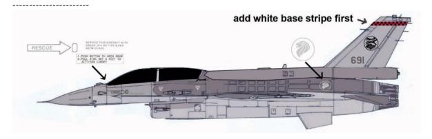
[A] F-16D Block 52-CF of the Singapore Air Force coded 691 of no.140 squadron "Osprey". It has the F100 engine with standard intake. Long thick spine fairing with probably systems and long tail base fairing.
