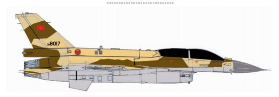
[B] F-16D Block 52 of the Morocco Air Force coded 08-8017. It has the F100 engine with standard intake. It has the long tail base fairing and full long thick spine fairing. Similar colours as for scheme [A].
