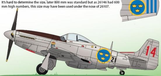
S 26, 26043, red 14 - F21. The last Mustang in the Swedish air force. Most likely dark brown antiglare panel. Last design of walkways, i.e. angled toward the gun ports, see topside view, both port and starbord wing.
