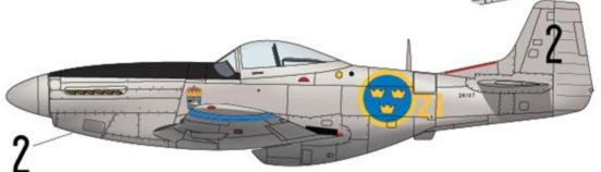
**S 26, 26107, 2 - F21Kallax/Luleå.** Three blue stripes were painted on the wing tips, top and bottom. The size of the stripes was approximately 120 - 150 mm wide. The a/c had earlier been equipped with an AN/APS-13 antenna. Most likely the call sign was painted under the nose instandard fashion.
