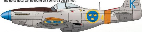
J 26, 26115, blue (most likely) Kalle - F4 Frösön/Östersund. Exercise markings in 1951, orange marking on fuselage and wings, top and bottom. Latest type of angeled walkways on wings.
