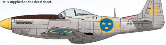
J 26, 26122, yellow Harald - F4 Frösön/Östersund. Straight walkways on left and right side. The aircraft had earlier been equiped with AN/APS-13 antenna from the time in 401 FS and the squadron code 9D was still visible on the airframe. It was common to paint (or use tape to mark?) the call sign on the landing light at F4. Not known if 26122 had it but suitible H is supplied on the decal sheet.
