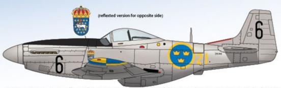
**S 26, 26146, 6 – F21 Kallax/Luleå.** Reconnaissance version of the J 26 with sKa10/50 camera in the fuselage. Call signs on both sides of the nose instead of underneath the nose which was standard. Blue and yellow fields on wing tips top and bottom. The spinner was painted silver done just like the
