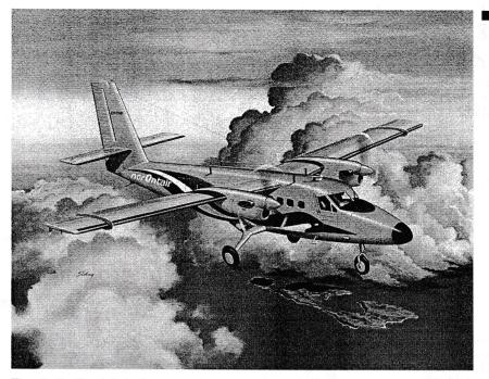
The de Havilland Twin Otter was designed in the early 1960s as the logical successor to its highly successful Otter. It improved on the Otter's design by including twin turboprop engines and tricycle landing gear. This enabled the Twin Otter to carry up to twenty passengers faster and more efficiently than any of it's short-haul competitors.
