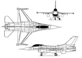
Even in the 2000's new F-16 variants were developed fitted with sophisticated avionics capable of firing and dropping advanced weaponry. Weights increased and beefed up gear and structures were needed. To increase range on some variants a pair of conformal fuel tanks CFT could be fitted on the mid fuselage section and to accommodate systems a thicker long spine fairing.
