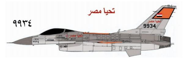
F-16C Block 40 of the Egypt Air Force coded 9934. It was delivered under the program "Peace Vector III" in the 1990s. It has GE F110 engine with bigger MCID intake.
