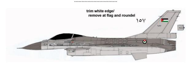
[B] F-16AM (MLU) of the Jordanian air force coded 157 (c/n 6H-120/M13-454 was the ex-Belgian F-16AM FA120). It has the Pratt and Whitney F100 engine with standard intake. IFF antennas on nose.
