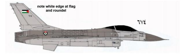
[A] F-16 ADF of the Jordanian air force coded 674, set in arab numbers. (ex-US ANG). (other codes also provided). It has the Pratt and Whitney F100 engine with standard intake. IFF antennas fitted on nose. Note ADF fairing at tail base (both sides) and short tail base without parachute housing.
