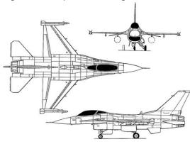
Even in the 2000's new F-16 variants were developed fitted with sophisticated avionics capable of firing and dropping advanced weaponry. Weights increased and beefed up gear and structures were needed. To increase range on some variants a pair of conformal fuel tanks CFT could be fitted on the mid fuselage section and to accommodate systems a thicker long spine fairing.
