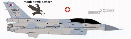
[C] F-16D Block 70 two seater of the Royal Bahraini Air Force coded 1612 serial 18-0012. It has the GE F110 engine with bigger MCID intake. It has advanced systems and thick long spine. Long tail base housing with extra ECM fairings.
