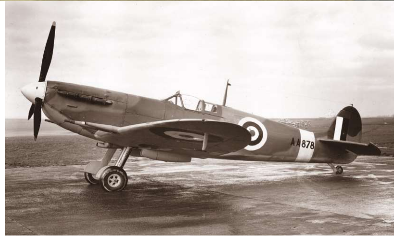
Spitfire Mk.Vc armed with four Hispano Mk.II cannons. Propeller is De Havilland, new canopy style with interior glass armor on the windshield and bulged sides of the canopy sliding portion. The aircraft supposedly carries an older type of radio Tr.9D.
