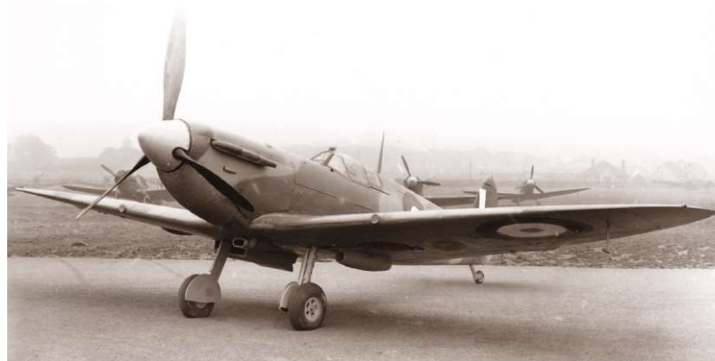
Early production Spitfire Mk.V manufactured in October 1941 with symmetrical lower bulges under the cannon well, enlarged cooler, older canopy style with exterior armor and hinged window hatch. The aircraft still lacks the armament, it's equipped with the De Havilland propeller and newer type of radio Tr1133.
