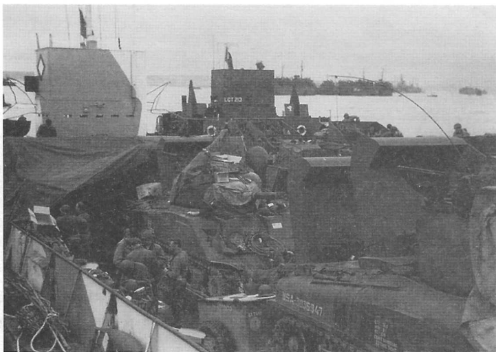
Sherman tanks on landing ships. Note the 'Snorkel' for air intake and engine exhaust. US Army photo.
