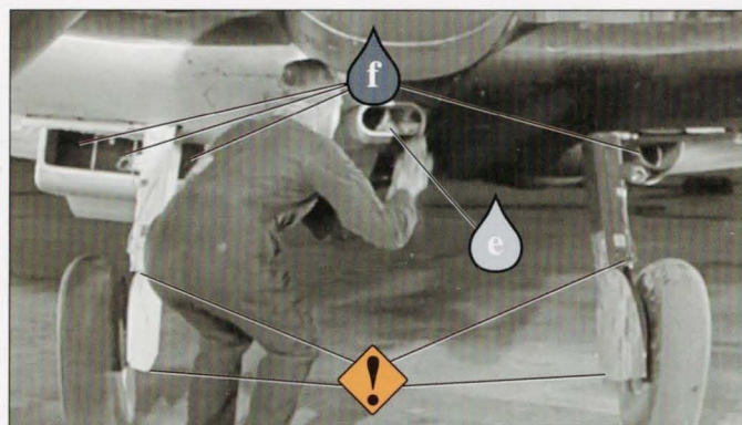
Undercarriage detail from late-production Spitfire Mk.Ia R6692. Note the carb air intake and uneven strut compression.
