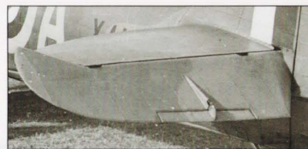
Port elevator detail from late production 616 Squadron Spitfire Mk.Ia X4172 or X4175 photographed on 26 September 1940. Note the hinge cutouts, subtle rib-stitching and lack of scalloping on the tightly doped fabric covered surface. Also note the lack of pre (and post) shading effects either side of the ribs.
