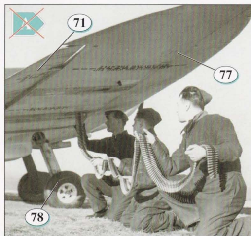
Early production 611 Squadron Spitfire Mk.I K9999 FY-D photographed on 11 January 1940. K9999 was completed in June 1939 when the undersides of the wings were being painted white and Night, with the underside of the fuselage painted aluminium. Note the factory applied stencils (71) & (77), Dunlop tyre marking (78) and the grease and cordite-stained gun access panels. The Spitfire Mk.I was rearmed from pre-loaded box magazines which were inserted into the wings from below, not from the romantically flowing belt presented here for the press photographer.
