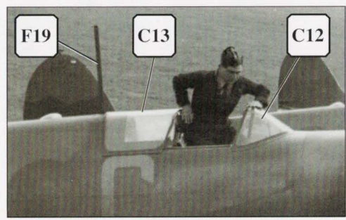
Spitfire Mk.I (K979#) WZ-C with unarmoured windscreen C12 photographed on 19 Squadron on 4 May 1939 still with its flat hood C13 fitted.
