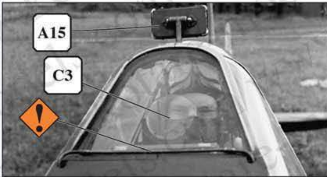
Windscreen detail from a Spitfire Mk.Va serving with 61 OTU in 1942. Note the horizontal tube for dispensing de-icing fluid, GM.2 reflector gun sight C3 and mirror A15 . The armoured glass windscreens on Spitfires in WWII were not tinted green like modern restorations.
