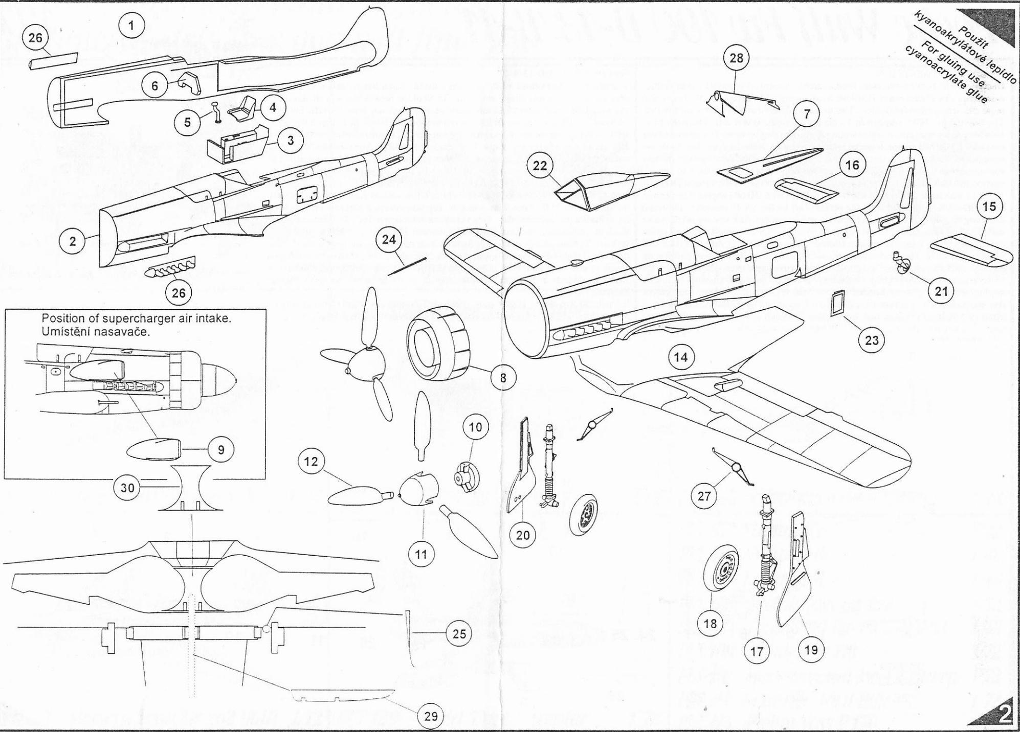
Position of supercharger air intake.
