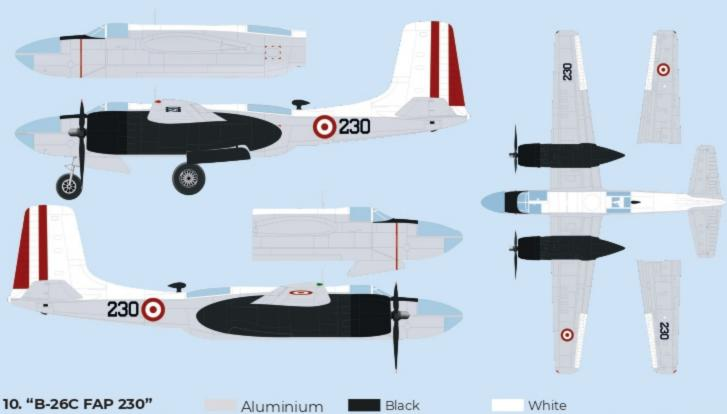
The B-26C serial FAP 230 was the last airframe of this type delivered to the Peruvian Air Force in 1960. Painted in aluminium with white upper surfaces and black engine nacelles and cowlings, FAP 230 was the only FAP Invader that wore a different paint scheme other than the standard black overall finish on these aircraft.
