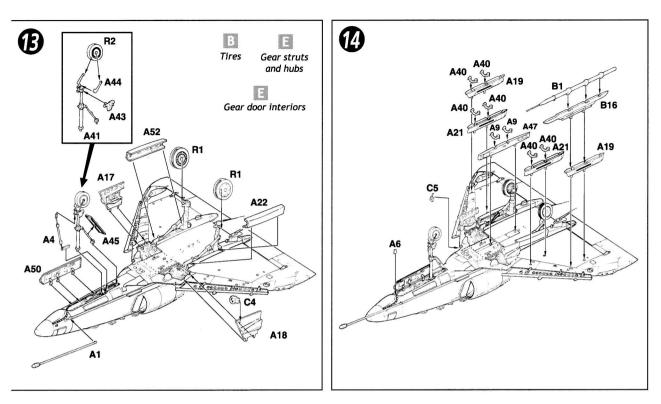
NOTE - Be sure to dry-fit and check alignment of all parts during assembly
