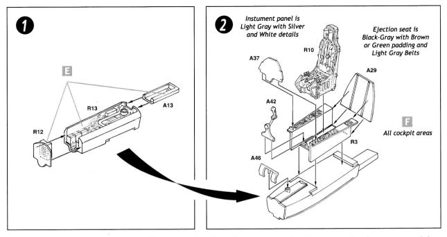
NOTE - Be sure to dry-fit and check alignment of all parts during assembly
