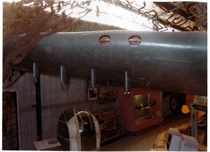
FIG 6. ROCKET MOUNTS - RIGHT WING
