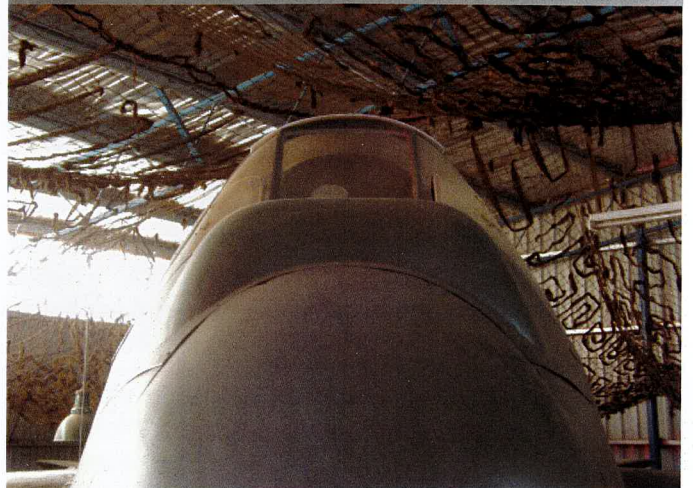
FIG 19. THE AUTOPILOT COVER FAIRING ON THE DAP MK 21
