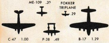
All Airfix 72 planes are made in 1/72 scale (1''=6'0''). For example, the M E 109 has a wingspan of  $5\frac{1}{2}$  while the B-17's is  $17\frac{1}{2}$ . Your entire collection will have the same relationship, ideal for collectors and enthusiasts. You can build over fifty constant scale combat planes in this series.
