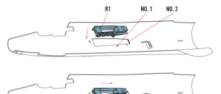
**3** AFTER THE PREPARATION OF SEATS IS COMPLETED, THE CONDUCTOR IS REMOVED AND PLACED IN HIS PLACE, USING THE SAME GUIDELINES, PART R3 IS INSTALLED
