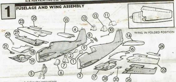
It is recommended that the instructions and exploded views are studied before assembly. Note that some parts are best painted before assembly. If stand is to be used cut away wall of plastic from stand slot in fuselage halves.
