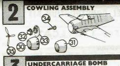
Select cowling for variant you wish to model, for F6F3 (30), for F6F5 (31), then cement forward radial engine half (32) to rear engine half (33), locating lug on top and front of rear engine half into cut out in recess behind forward radial half.
