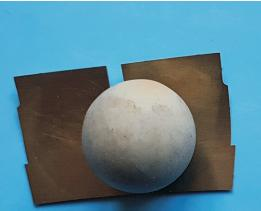
Form the PE splitter plate with a rubber ball or similar.
