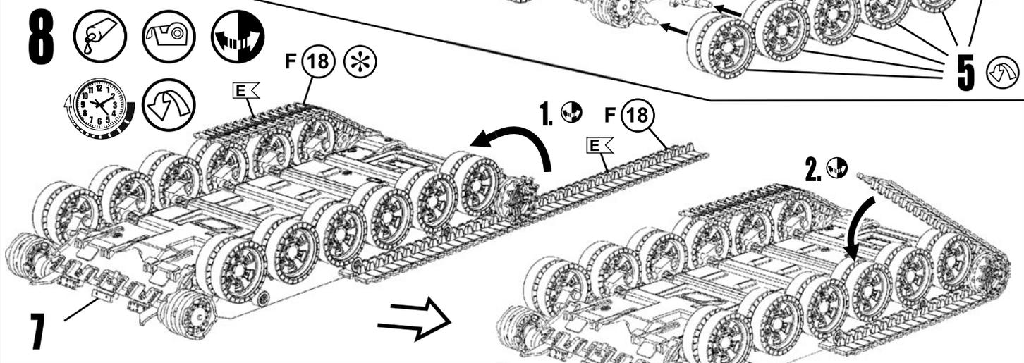
Bend with the help of hot water, do not use boiling water in any case!
