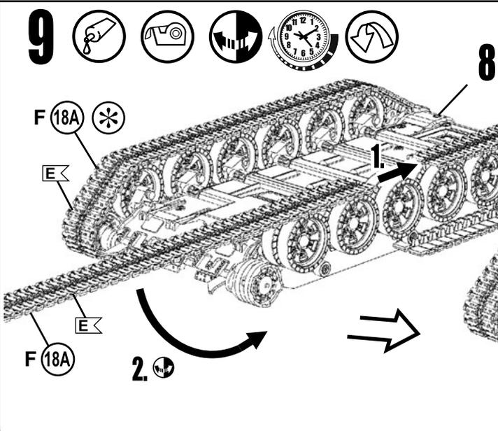
Bend with the help of hot water, do not use boiling water in any case!
