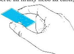
5. Lightly place the component in the desired location and position. Adjust as required. The component will be permanently affixed when pressed onto its intended location, its location can be adjusted.
