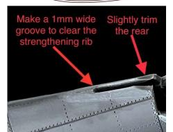
■ Tail Post: With the original tail chopped off, all left is to remove material to allow for the strengthening rib on the tail post. Width of the rib is 1mm length is 11.6 mm. Check fit regularly
