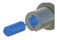
Insert motor into the front plug, be careful to push it to the front lip (lip is fragile). Mind the wiring output must be horizontal to allow clearance for the motor rear fix. Avoid pushing on the wires while inserting.
