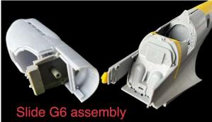
slide G6 assembly into the nose, don't glue it immediately
