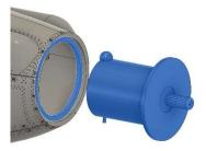
Insert motor into the front plug, be careful to push it to the front lip (lip is fragile). Mind the <u>wiring output must be horizontal</u> to allow clearance for the motor rear fix. <u>Avoid</u> <u>pushing on the wires while inserting.</u>
