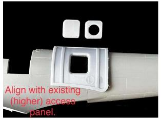
Retractable Tail Wheel: Start with the LH side template, it slots into the rudder actuator recess on the fuselage. Fix it with tape, then fix the RH side template at the exact same height. Once happy, proceed with razor saw, scalpel and finish with flat file.
