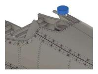
Insert magnet 3 with the marked face inside in the nose part.
