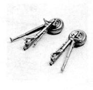
Cement landing gear assemblies into main gear wells, then cement D7 and D8 to bottom edge of wing next to wells.
