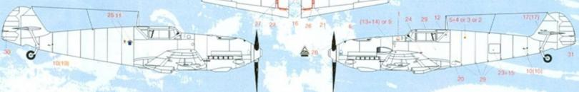
Standard Factory Stencils for the early BF-109 B-C-D-E Family. Take into consideration that not all were used on operational A/C. specially after Field repairs and painting.
