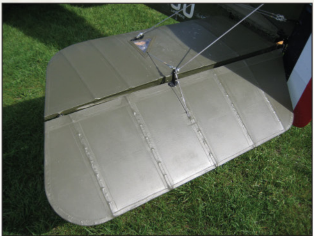
Tailplane and elevator from WA19, note the clear pulley inspection panel and prominent rib tape stitching.
