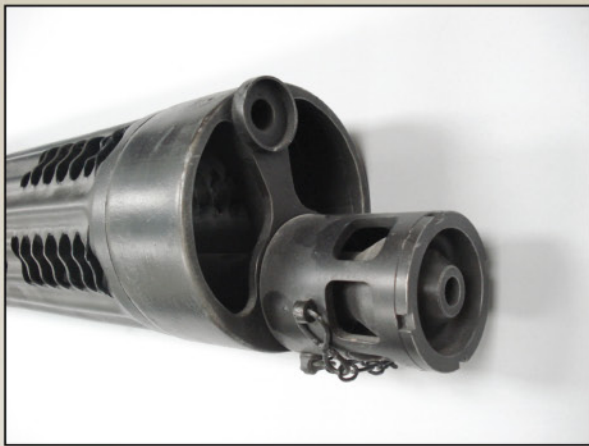
Vickers Mk.1* showing the brass breech block, muzzle details and air vents cut into the cooling jacket. Note that this gun features a Hyland type B loading handle of a different design to the Hyland type E commonly fitted to the SE.5a and featured in our model.
