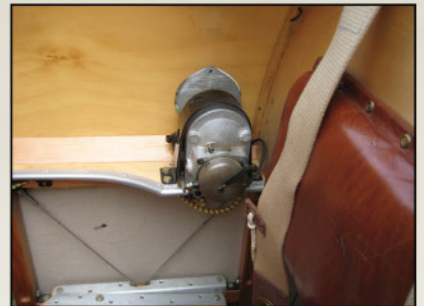
Magneto starter located to the right of the pilot's seat.
