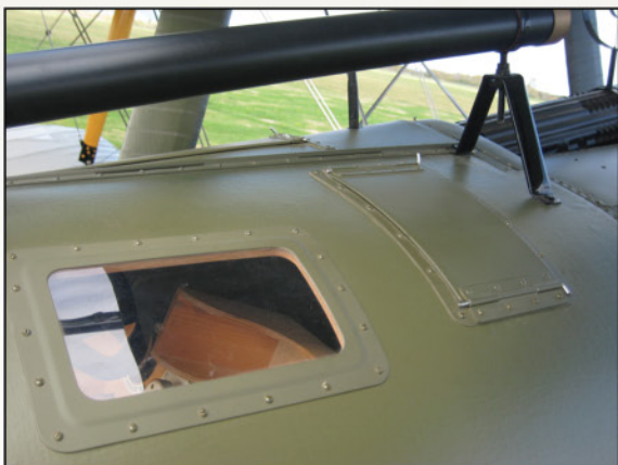
More detail from WA19 showing Aldis sight front mount, Vickers gun magazine hatch and window to help illuminate the instrument board.
