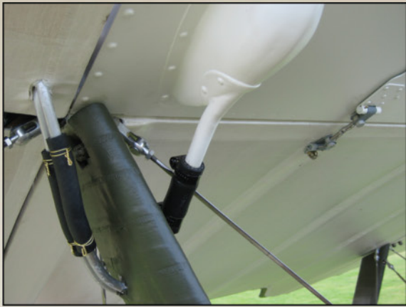
Starboard front cabane strut showing wing fuel tank sump 'bubbles', and fuel line and pitot tube pipes entering the fabric wrapped strut.
