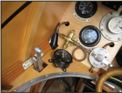
Instrument board of TVAL WA19 showing colour details of the instruments and control column. Note bare metal edging to the cockpit stiffener and the difference between the linen fuselage panel sides and plywood cockpit coaming.
