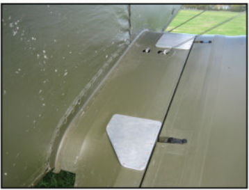
< Foot steps and lower wing root, note the wing attachment brackets.
