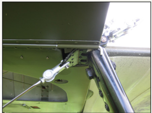
Rigging details at top of front left strut.
