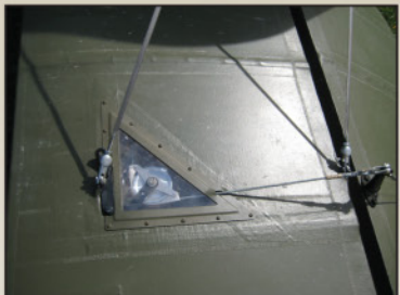
Elevator control cable pulley inspection panel detail from tailplane.
