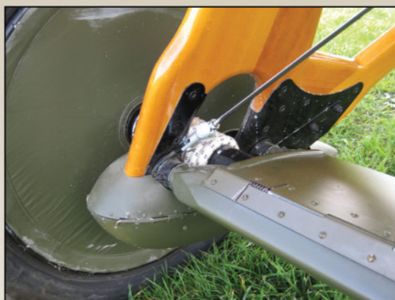
Detail from WA19 showing late style wooden undercarriage legs with bungee cord bullet fairing. >
