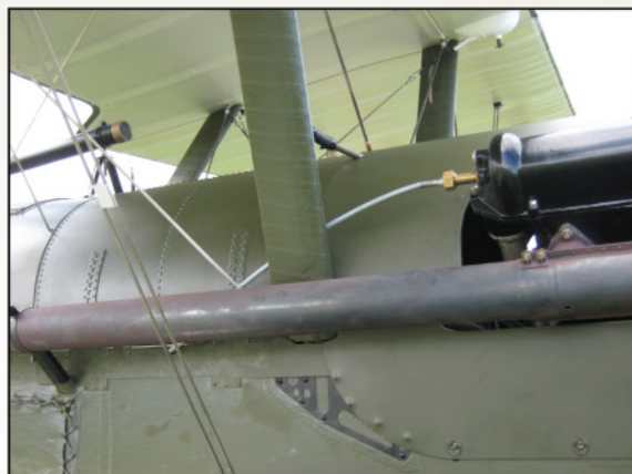
Note the fuel tank details, various brackets and fabric wrapped cabane struts visible in this shot of WA19. This aircraft is powered by a genuine Hispano-Suiza engine, though it is one of the direct drive types and doesn't have the fairing details of our geared engine model.
