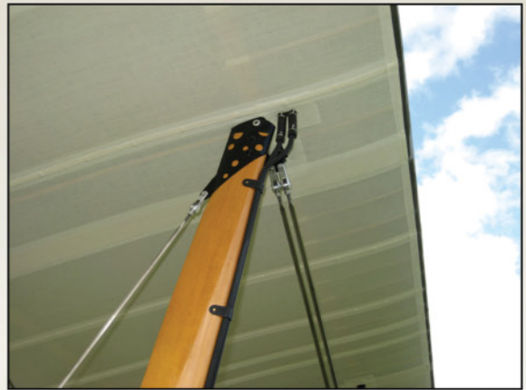
Front starboard wing strut showing Pitot tube with leads running into the upper wing, strut end bracket and double RAF wire.
