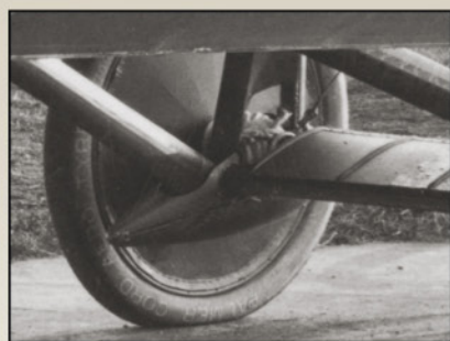
< Detail from B4897 showing an early attempt to strengthen the steel undercarriage, Palmer Cord Aero tyre and bullet shaped bungee cord fairing.
