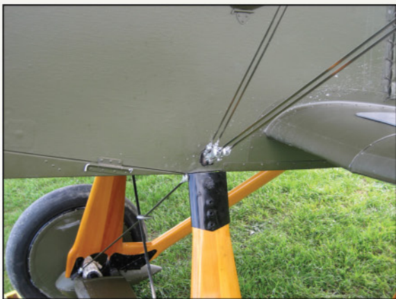
Undercarriage front strut attachment bracket. Note the two pairs of RAF flat profile rigging wire.
