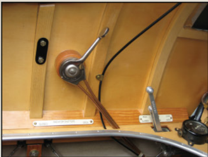
Throttle and radiator shutter control levers (in line engine type).
