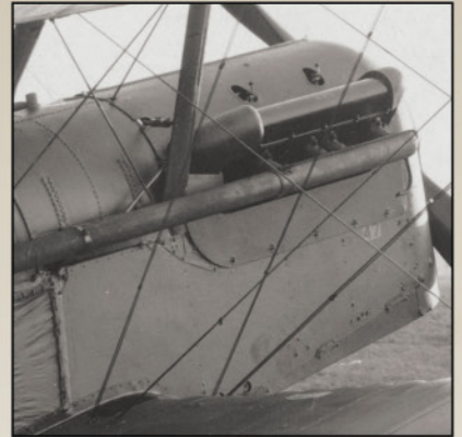
Nose detail from B4897 showing round cutouts in the cowling for the engine priming cups and rigging details.
