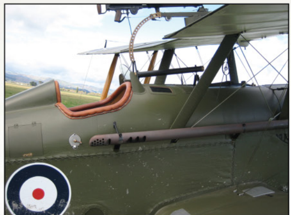
Exhaust detail from WA19. Note the subtle variations in the cockpit padding and windshield fairings from B4897.
