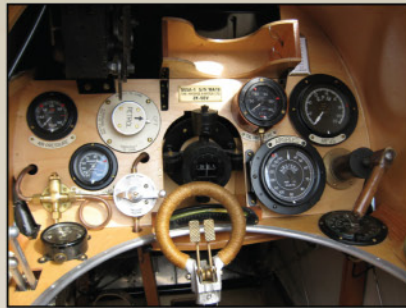
Instrument board of TVAL WA19 showing colour details of the instruments and control column. Note bare metal edging to the cockpit stiffener and the difference between the linen fuselage panel sides and plywood cockpit coaming.
