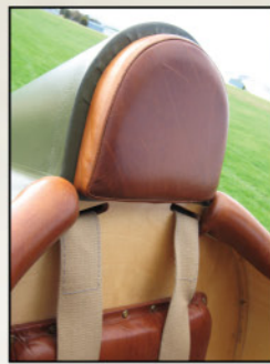
Headrest showing leather padding details. Note the four point Sutton safety harness, not usually seen on wartime aircraft.
