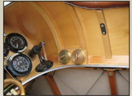
Instrument board of TVAL WA19 showing colour details of the instruments and control column. Note bare metal edging to the cockpit stiffener and the difference between the linen fuselage panel sides and plywood cockpit coaming.
