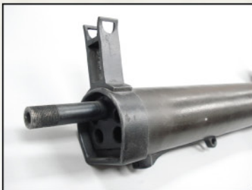
Note the holes in the end of the lightened casing to aid the flow of air to cool the barrel.
