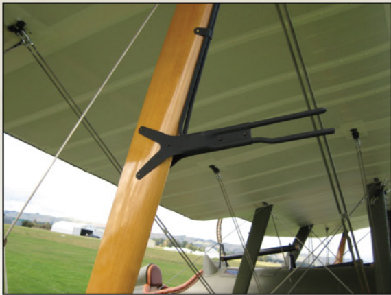
Front starboard wing strut showing Pitot tube with leads running into the upper wing, strut end bracket and double RAF wire.
