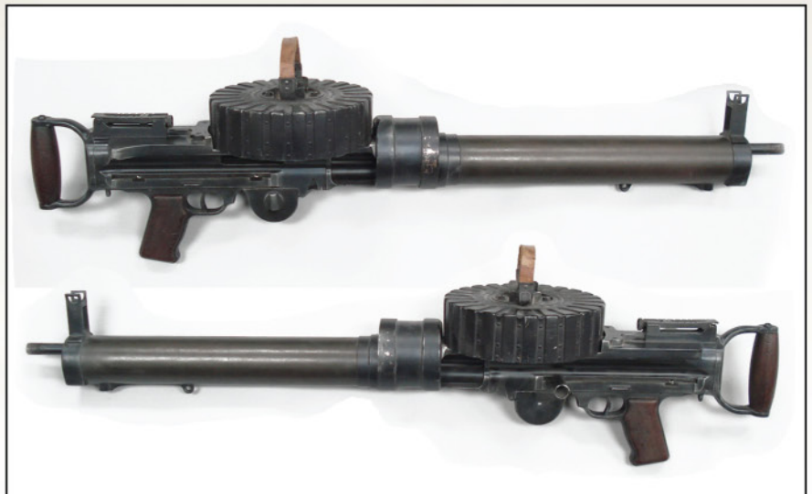
Lewis Mk.II (RFC pattern with lightened barrel casing). Note the dark wooden hand grips and the leather strap on the 97 round drum magazine.
