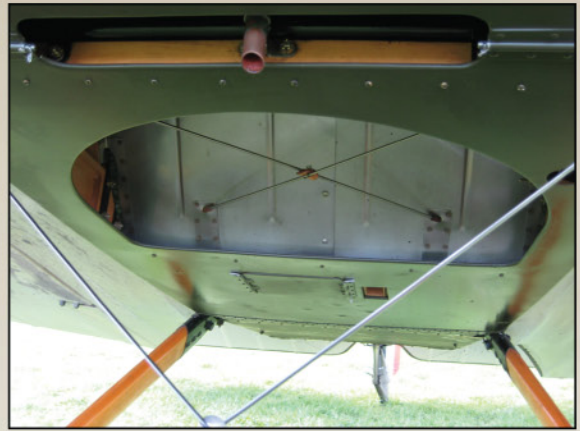
Underside view showing rear undercarriage strut attachment brackets, late Viper style baffle plate (firewall) and exit port for spent Vicker gun cartridges.
