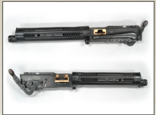
Vickers Mk.1* showing the brass breech block, muzzle details and air vents cut into the cooling jacket. Note that this gun features a Hyland type B loading handle of a different design to the Hyland type E commonly fitted to the SE.5a and featured in our model.
