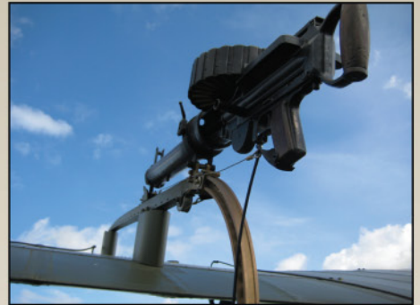
Foster mount and Lewis gun from TVAL WA19. While WA19 is direct drive powered, it retains the raised Foster mount of a geared engine SE.5a. Many direct drive SE.5a continued to be equipped with raised Foster mounts, even though they no longer required the spacers.
