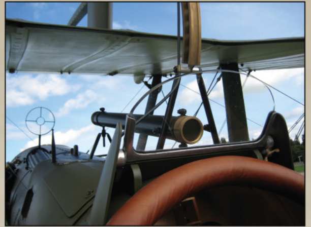
Aldis sight and windscreen details from WA19. Note the brass ends of the Aldis optical sight, the ring and bead sights and method of attaching the Foster mount brass rail to the Aldis sight bracket.
