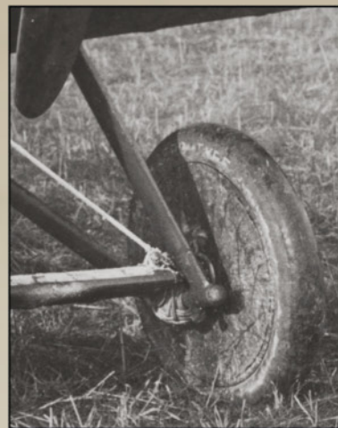
Early steel undercarriage leg from C1057. The bullet shaped bungee cord fairing has been removed, possibly to prevent an excessive build up of mud restricting movement.
