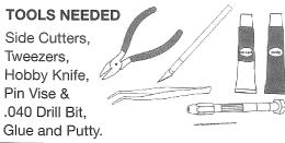
For best results, read this sheet COMPLETELY before assembly! Dry fit parts before paint and assembly, use tube type styrene glue or styrene solvent, never use cyanoacrylate glues! See build video tips at salvinosjrmodels.com/videos.
