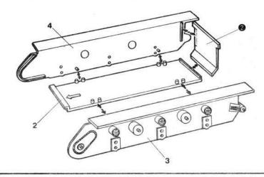
Cement assembled bogies to hull sides as indicated. Cement two 14's to round pads on each side. Cement 8 and 9 together then to rear pins on hull, one set to each side. Cement 6 and 7 together then cement one set to forward pins on each hull side. Cement 1 to top of assembly then cement 16 to the hull front.
