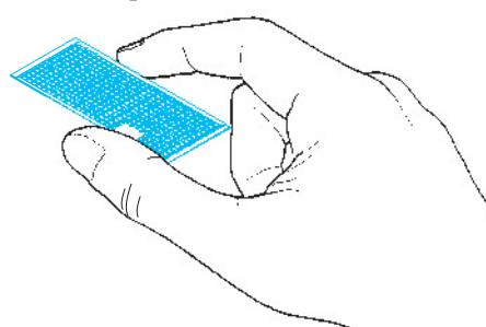
5. Lightly place the component in the desired location and position. Adjust as required. The component will be permanently affixed when pressed onto its intended location, its location can be adjusted.
