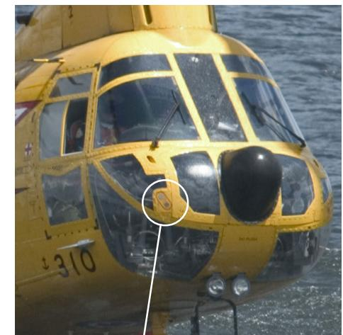
Above left, the Labrador (post-SARCUP with radome). Right, the ex-Voyageur CH-113 Labrador. Note that starboard outboard clear panel has a small corner extension which is NOT present on the other side.
