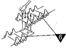
\* Melt pins together with a heated screw driver.
