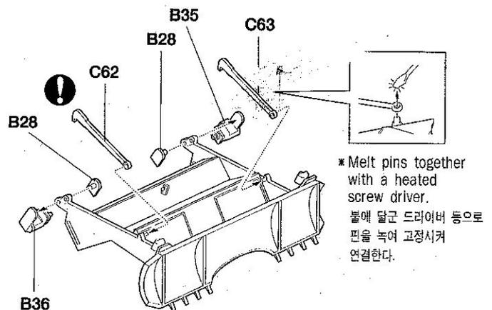
\* Melt pins together with a heated screw driver.
