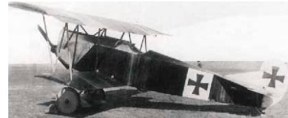
An early Fokker D.VII with Mercedes D.IIIa engine in the typical Fokker streaked finish (Albatros/PL Gray Collection-used with permission)
