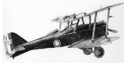
British SE 5a, powered by Wolseley W.4A Viper 200 hp engine, max. speed 222 km/h
