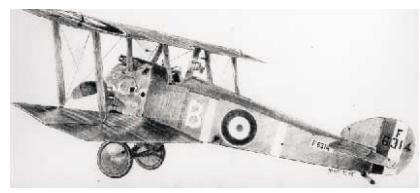
British Sopwith Camel, with Clerget 9B 130 hp engine, max. speed 185 km/h.
