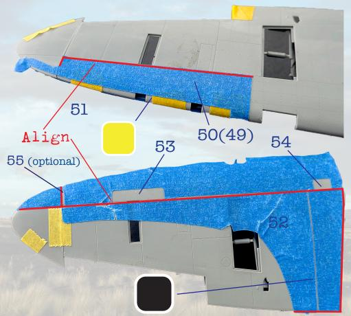
Note: use open squares in mask 52 as windows to align walk-ways above the wing spar, then mask with 53 and 54.
