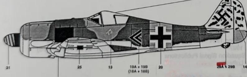
Fw-190A-6, I./JG 54, flown by Lt. Walter Nowotny, Eastern Front, 1943. RLM 74/75/76 camouflage with overpainting in two shades of green on upper surfaces. Yellow fuselage band, lower wingtips and bottom of rudder. Black spinner with white spiral. References on this aircraft vary considerably. Consult references to draw your own conclusions on colors.
