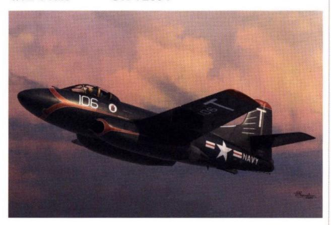
Douglas Aircraft received go ahead from the Navy for its F3D Skyknight in April 1946. The Skyknight was to be a two-seat, twin-engine, carrier-based night fighter. It had two radars in the nose, one for search and one for aiming its four 20mm cannon without requiring the target to be in sight. A rearward-facing radar was also installed in the tail to warn the crew of an attack from behind. The crewman in the right seat operated the radars while the pilot in the left seat flew the airplane.
