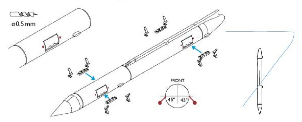
Before using, the parts should be washed with dishwashing detergent and primed with spray primer. Light sanding may be needed to remove 3D print strata marks.
