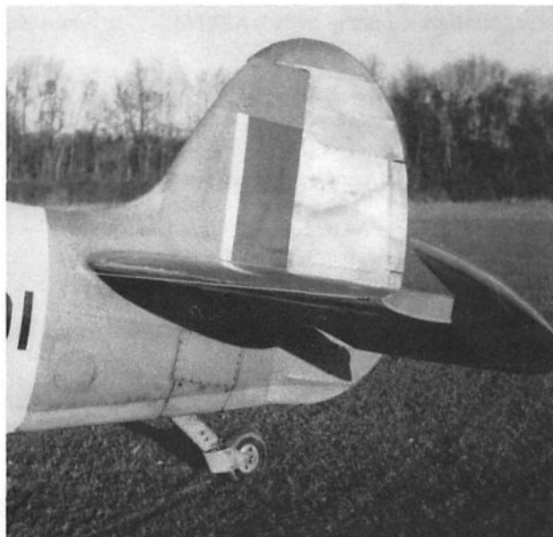
Additional details of the tail section can be seen from the left side. This particular aircraft does not have the usual mount for the radio antenna wire at the top of the rudder.
