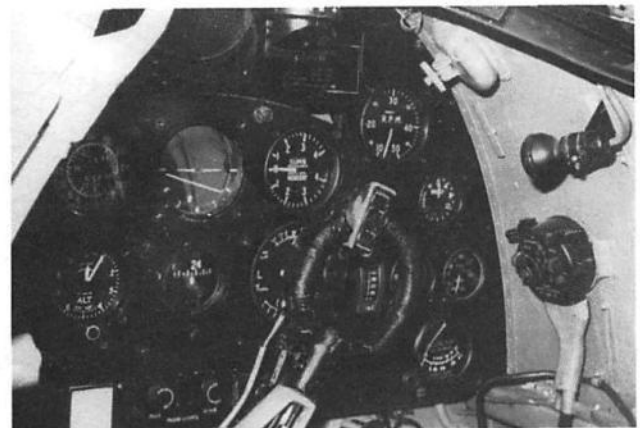
Details of the instrument panel can be seen here. Note that the circular handle at the top of the control column was wrapped tightly with black tape.
